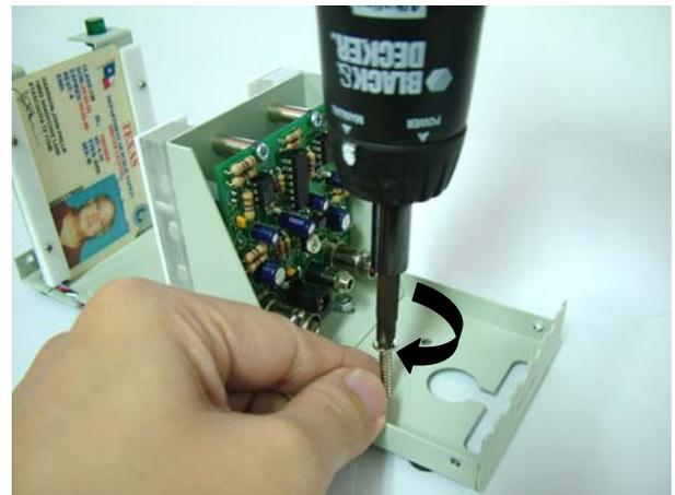
**Step A5** Use the base cover assembly as a template to mark the holes at the location to be mount.
