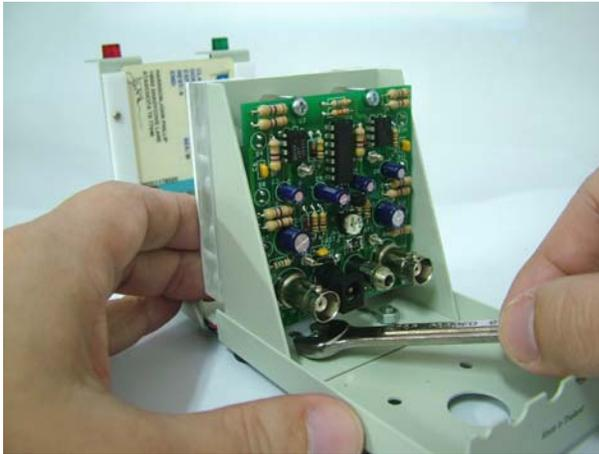
**Step E1** Use a spanner size 7mm to loosen the two hexagonal nut on the slide plate.
