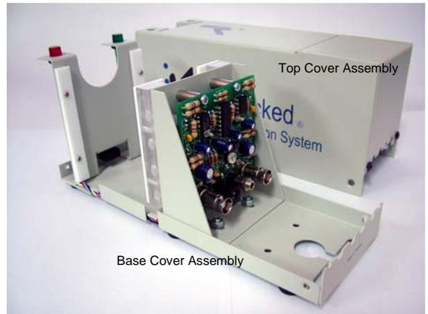
**Step A3** Slightly pull the base cover and push the 2 LED from the top side to disengage the base from the top cover.
